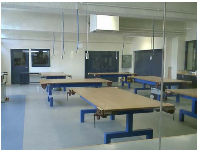
Workshop – benches, safety area, air & power overhead
